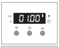
When the time has elapsed, the function indicator flashes and an audible signal sounds for 2 minutes.
